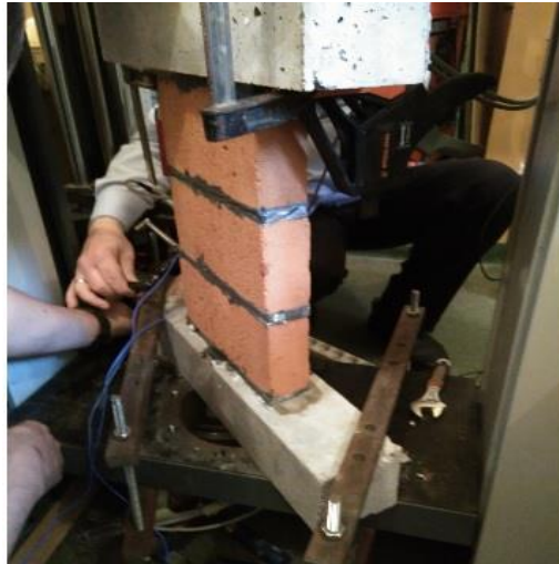
Figure 6. Tested specimen of dynamic test with polymer between bricks and and epoxy between bricks and concrete.
